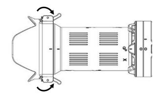
3. Lock the shade by pushing the locking levers downwards.
