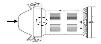
2. Align the lens alignment mark on the shade to the shade alignment mark on the objective lens and then push it in.
